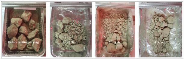
Figure 7- The change of disintegration in marl sample after slake index test depending on the number of cycles (L10-1).
