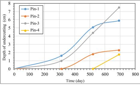
Figure 6- The time-dependent change of the depth of undercutting in pins installed in L1 due to effective weathering processes at natural conditions.
