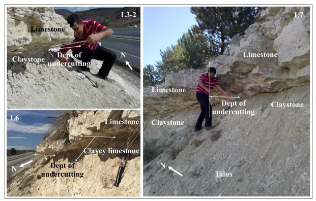
Figure 4- Measurements of the undercutting depths taken in road slopes with known excavation dates.
