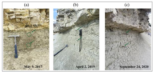
Figure 5- The undercutting depth measurements for location 3-1 using steel pins and screws; a) removing of the disturbed parts where the measures would be taken, obtaining fresh surfaces and installing pins, b) and c) the depth of undercutting observed in the pins on different dates.
