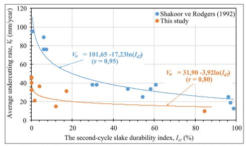
Figure 9- The relationships between average undercutting rate values and second-cycle slake durability index values obtained in this study and studies carried out by Shakoor and Rodgers (1992).
