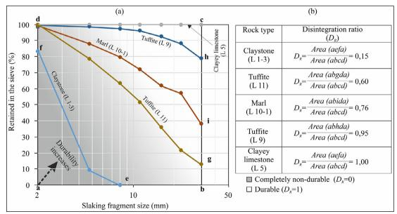
Figure 8- a) The fragment size distribution curves of clay-bearing rocks after the slake index test and b) the calculation of the disintegration ratio for the clay-bearing rocks (Ergüler and Shakoor, 2009).
