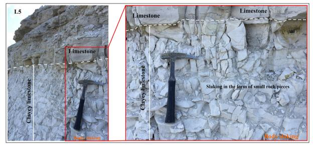
Figure 10- A typical example of the body slaking behaviour in clayey limestones in the form of small rock pieces in atmospheric conditions (L5).
