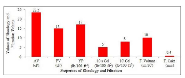
Figure 4- Rheological and filtration properties of drilling fluid containing NaCl saturated drilling fluid preparation water + XCD + PAC L + modified starch (F. Cake: filtrate cake).
