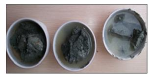
Figure 7- Keeping the core samples in mud and water and observation of the properties such as dispersion and swelling.
