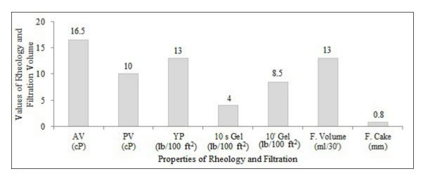
Figure 3- Rheological and filtration properties of bentonite + modified starch + XCD based drilling fluid.
