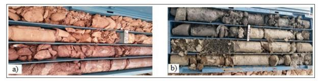
Figure 1- a) Brittle mudstones encountered in the Terzili and Yörüklü areas and b) unconsolidated sandstones, claystones and siltstones in the Suluova field.
