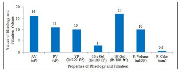
Figure 2- Rheological and filtration properties of bentonite + HV CMC + LV CMC based drilling fluid.
