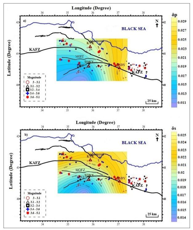
Figure 9- Obtained from the station; a) op regional absorption coefficients, and b) the lateral tomography of os regional absorption coefficients. NAFZ: North Anatolian Fault Zone, MOFZ: Merzifon Ovacık Fault Zone, EPFZ: Ezinepazarı Fault Zone.
