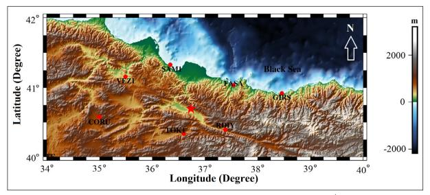
Figure 4- The view of the CORS-TR stations located near the epicenter (Erbaa district of Tokat province) of the 9<sup>th</sup> October 2015 ( $M_L$ =5.1). Red dots: the locations of GNSS stations of CORS-TR, red star: the epicenter of the 9<sup>th</sup> October 2015 ( $M_I$ =5.1) earthquake.
