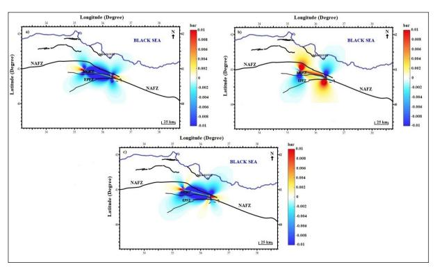
Figure 2- a) Shear stress, b) normal stress, and c) Coulomb stress values calculated by the earthquake focal mechanism data of KOERI (blue color: stress release, red color: stress loading).
