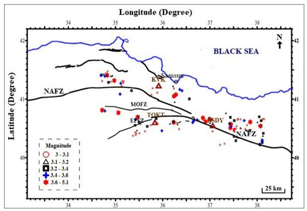
Figure 7- The locations of the stations (KVK, TOKT, RSDY) and the distribution of earthquakes used in the absorption analysis. Burgundy triangles represent the locations of the stations. NAFZ: North Anatolian Fault Zone, MOFZ: Merzifon Ovacık Fault Zone, EPFZ: Ezinepazarı Fault Zone.
