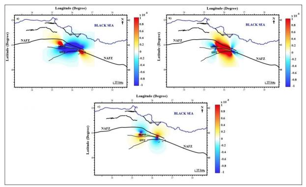
Figure 3- The strain a) XX, b) YY, and c) ZZ component variations calculated by using the earthquake focal mechanism data of KOERI.
