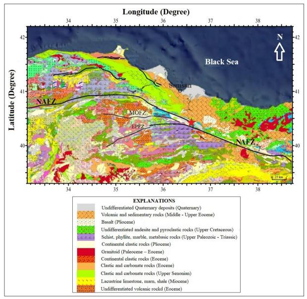
Figure 1- General tectonic and geological structure of the study region and its surroundings (modified from http://yerbilimleri.mta.gov.tr/ anasayfa.aspx). NAFZ: The North Anatolian Fault Zone, MOFZ: Merzifon Ovacık Fault Zone, EPFZ: Ezinepazarı Fault Zone. The red star represents the epicenter of the earthquake that occurred on October 9th, 2015 (M<sub>1</sub>=5.1).
