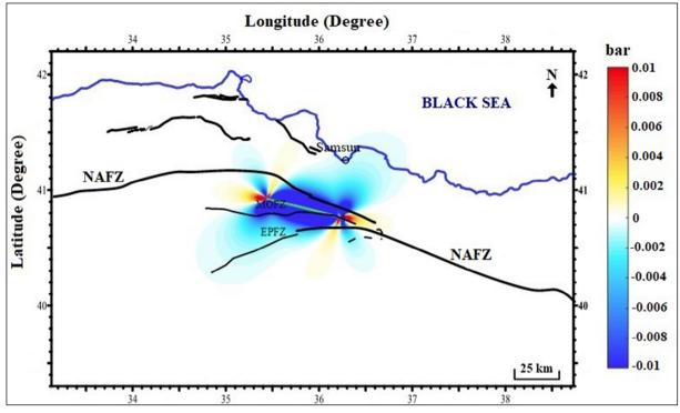
Figure 10- Coulomb stress changes on the study field. NAFZ: North Anatolian Fault Zone, MOFZ: Merzifon Ovacık Fault Zone, EPFZ: Ezinepazarı Fault zone.
