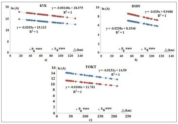
Figure 8-  $\ln(A) - \Delta$  (km) graphs and Pg - Sg absorption values of the stations; a) KVK, b) RSDY and c) TOKT.
